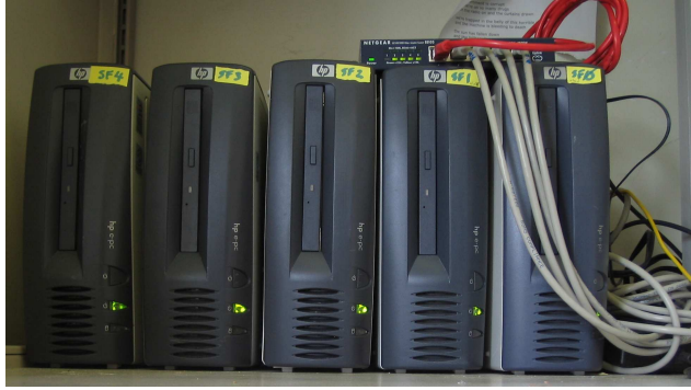
Figure 7: A five PC cluster over which the distributed simulation infrastructure was deployed.
